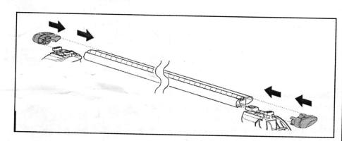
1) Use a flat-blade screwdriver to twist the lock plug, and remove the covers.
